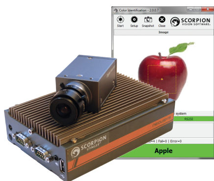
Scorpion Ultra Compact PC with camera and Scorpion Vision Software®.
