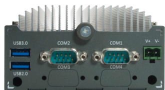
Rear view - 12 volt pwr - 2 rs-232 ports - 2 USB ports - power input
